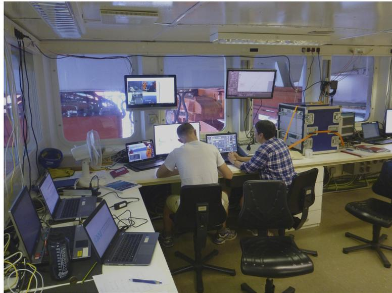
Fig. 3.7: Triaxus control centre with deck unit (blue box) and various laptops for running the steering software and programmes for data acquisition, rigged up in the Scientific Working Room II of Polarstern, which deigns a look to the aft deck where the winch is placed (Foto: V. Strass).
