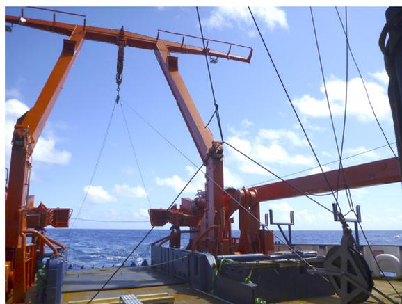
Fig. 3.6: Towing cable path and guiding over the aft deck; the turning block next to the winch container is seen in the bottom right corner (Foto: V. Strass)
