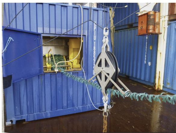
Fig. 3.5: Winch with towing cable in its container housing (Foto: V. Strass)
