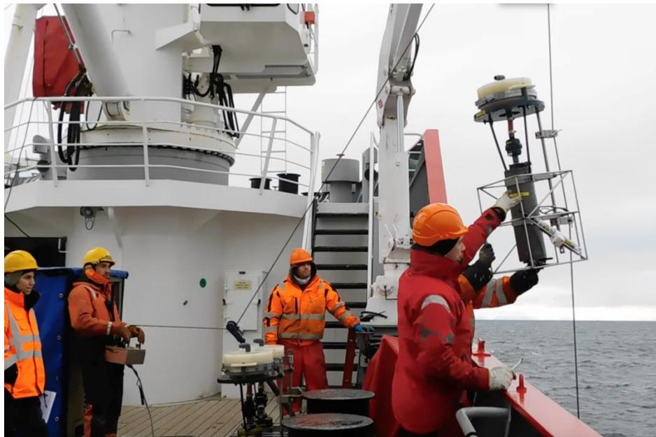
Normally the SAPs were deployed concurrently with the CTD, except in heavier ice conditions when the wires were worked separately. The ballast weight was always deployed and veered to 10m before starting the SBE39plus loggers and starting the SAP timer sequence. The period from starting the SAP timer sequence to having all SAPs at their target depths was approximately 30 minutes. Recovery from start of haul to all inboard was approximately 15-20 minutes.
