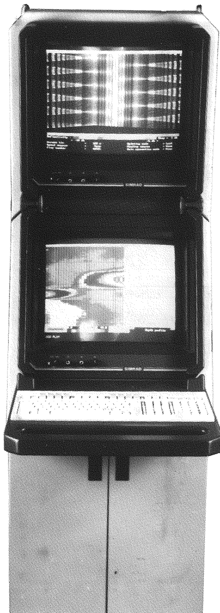
Figure 6 The dual height display console for the Sonar Imaging and Quality Assurance Units
