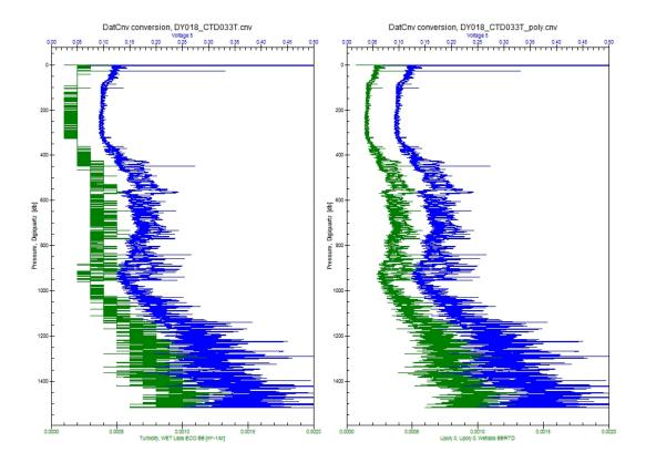
(4) Manual identification of the surface soak (while waiting for pumps to turn on) and the end of the downcast using the 2Hz files. Times to crop were saved to JC105\_ castcrop\_times.mat.
