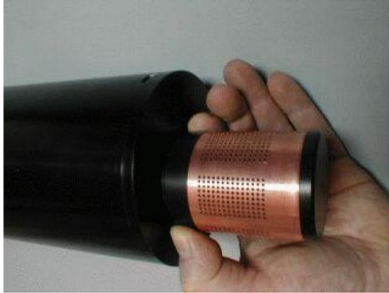
*Figure F-9: Mounting the guard*
